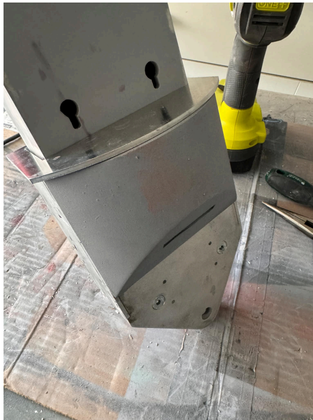
Finished ankle attached to leg (with 3D-printed beefy part attached)
