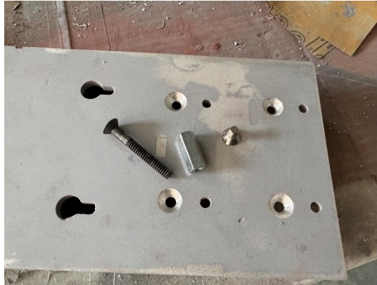
Parts needed for couplers and the four locations on the leg to countersink
