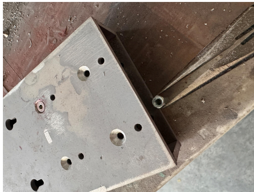
Using needle nose pliers to assist in attaching M6 couplers
